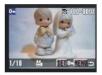
5. Press the Set button (SET) to protect( ) the picture or press the"MENU" button to cancel ( MENU ) this protection and return to the main menu.
